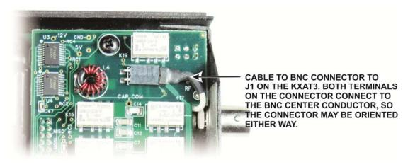
Figure 6. Connecting Antenna Plug to KXAT3 Board.
