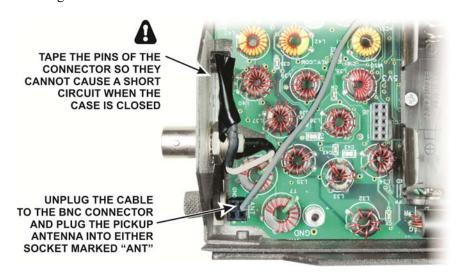
Figure 3. Connecting the Test Antenna to the KX3 Input - No KXAT3.
