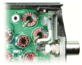
Figure 5. Connecting the Antenna Plug to the RF Board - No KXAT3 Installed.
