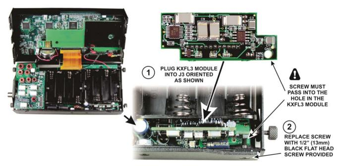
Figure 1. Installing the KXFL3 Module.
