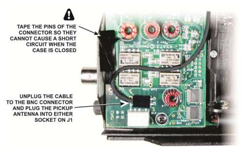
Figure 4. Connecting the Test Antenna to the KX3 Input – With KXAT3.
